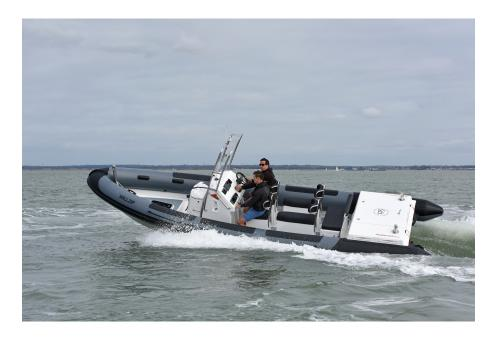
These boats are built to deal with rough seas with their moulded splashwell at the stern, providing increased structure and ensuring the safety of crew onboard the vessel. Island RIBs fit hand moulded polycarbonate windscreens rather than the industry standard acrylic. These windscreens are completely shatterproof and coated to provide UV protection.
